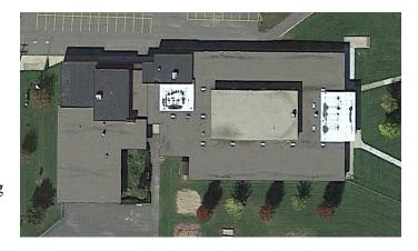
A renovation has recently been completed that include installing HVAC units and conduit that rest directly on the roof membrane. Based on our field observations and core cuts, there are four different roof systems/eras of construction present. Our Field Observations, Conclusions/Recommendations and Budget Forecast is separated per each roof system.
