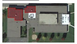
The existing roof system with these sections consists of a 90 mil fully adhered EPDM membrane. The roof appears to be recently installed and is likely covered under a manufacturer's warranty. Based on this no core was taken. Drainage is accomplished via tapered insulation to internal roof drains with either adjacent overflow drains or scuppers. The total of all roof sections was 5,462 Square feet. Refer to photographs #24 and #25 for overviews of the roof areas.
