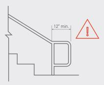
Not providing ADA compliant railings at stairs
