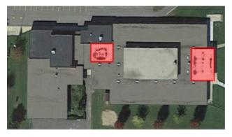
The roof system within these sections consisted of a coated EPDM membrane. A core sample take within Section 2 indicated that the EPDM roof membrane was installed over 2" polyisocyanurate insulation, 1 ½" wood fiber insulation, an asphalt vapor retarder and a concrete roof deck. Moisture was observed in the insulation at the core location. (Refer to photograph #17).
